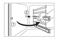
Installing the shelf support rails
